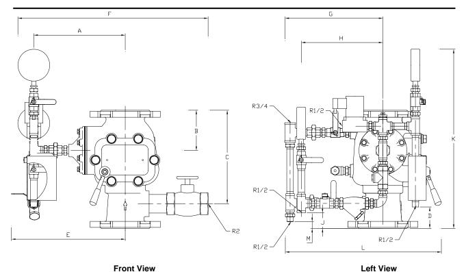
Nominal Installation Dimensions in Inches and (MM) VALVE В С D Κ Α L Μ SIZE 11.3 4.96 11.54 2.71 14.05 23.5 12.09 10.08 1.97 22.05 19.3 0.87
